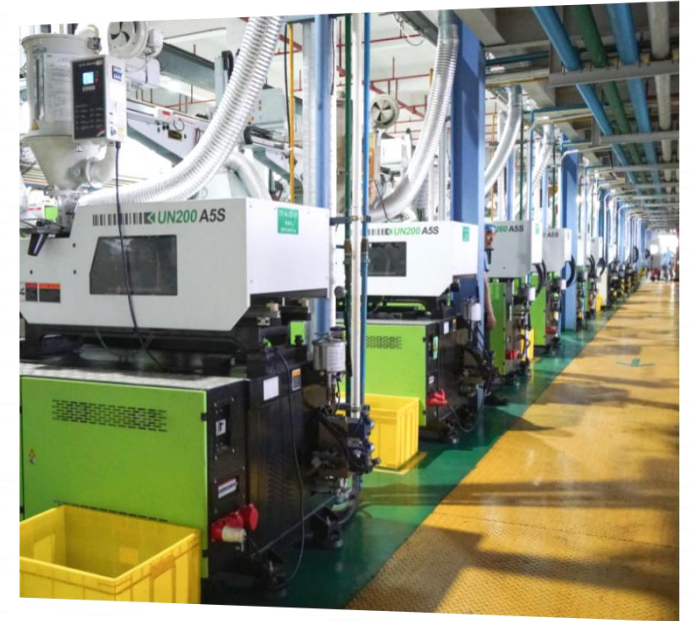
● Injection Molding with Central Material Feeding System (Raw materials are separated from the production site)
